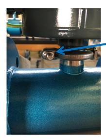
Partially unscrew the nut of the clamp that connects the converter to the sensor
