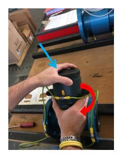
keep still the top of the housing (blue arrow), and unscrew the aluminum base that will rotate within the clamp (red arrow)
