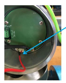
Connect the battery pack to the 5 way connector.
