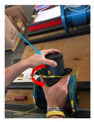
Hold the housing, screw the aluminum base and then fix the clamp
