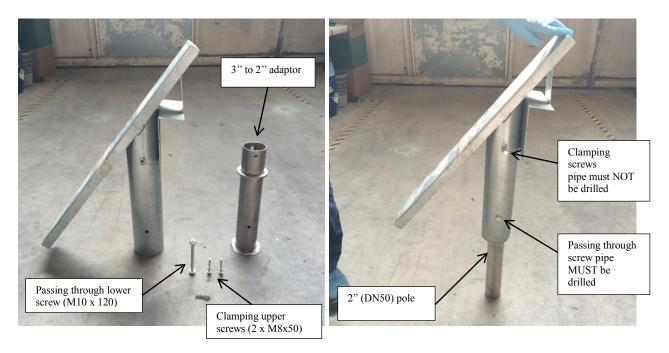
6- Once the solar panel is oriented in the right direction tight the bolts on upper side of the bracket to the pole to avoid rotation of the panel, drill the pole in order to fit the lower passing through screw and tighten it, in order to avoid any long term unscrewing.
