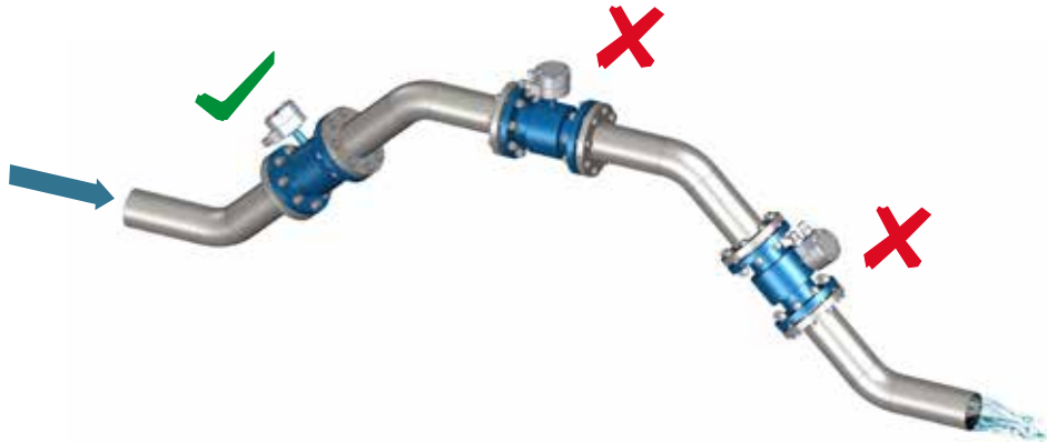
Fig. 21 Correct (LH) and incorrect installation (central and RH)
