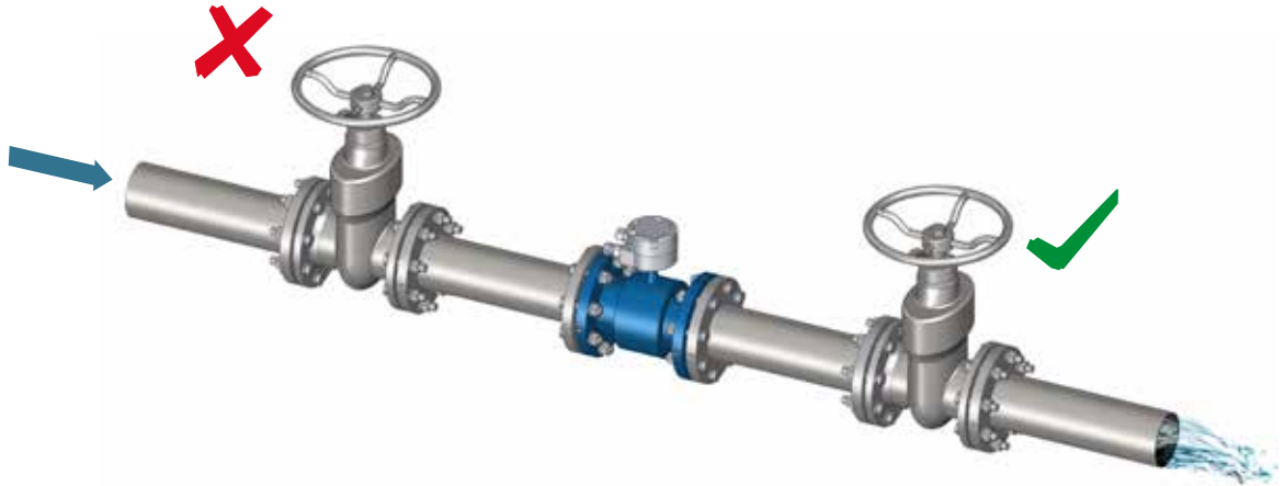
Fig. 22 Gate valves installation
