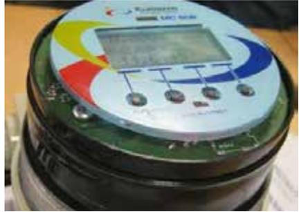
2. Carefully remove the front board support .
